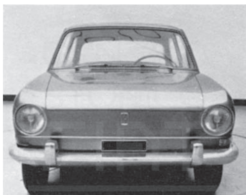
The coachwork of the G. 123 E2 was a compromise between two and three volumes. The rear position of the engine and the particular type of cooling allowed the front grille to be eliminated.
