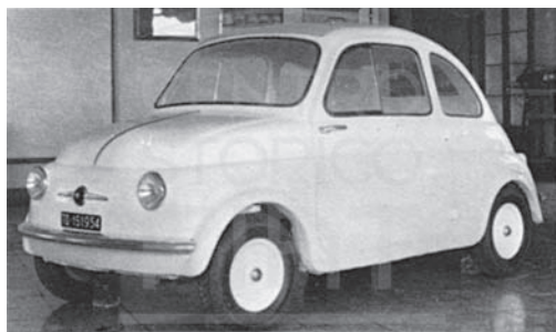
Full-scale plaster mock-up of the 110-518, a coachwork design for the Nuova 500, August 1954.
