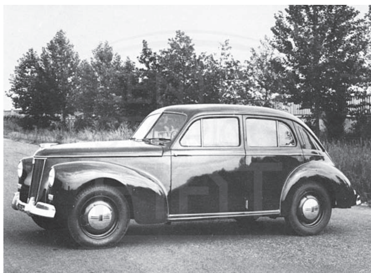
Working prototype of the “101 E1” sedan, whose chassis foreshadowed many elements of the final design adopted for production of the 1400. Photos taken the 15 October 1946.
