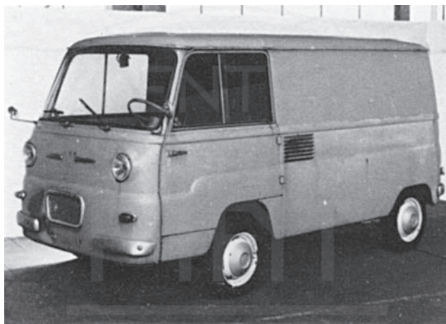
The front-wheel drive 02 van was built at Heilbronn under Cordiano. The Fiat 500 motive unit, shifted to the fore carriage, had the engine at the back of the two seats.
