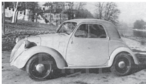
The 500 B was practically indistinguishable from the Topolino first series, except from minor details such as the clamps of the radiator grill.
