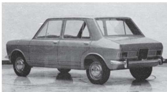
The shape of the “X 1/1” (the future 128) constructed to the instructions of the author lent itself to the addition of a hatch at the rear.
