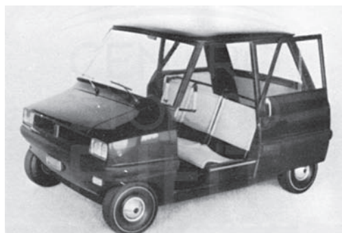
Studies were also made at SIRA of city cars. This design, dated 8 June 1963, is a variant (study 794) for the G. 26/518 small car. The G. 26 was revived in 1964 as the basis for a small electric auto.
