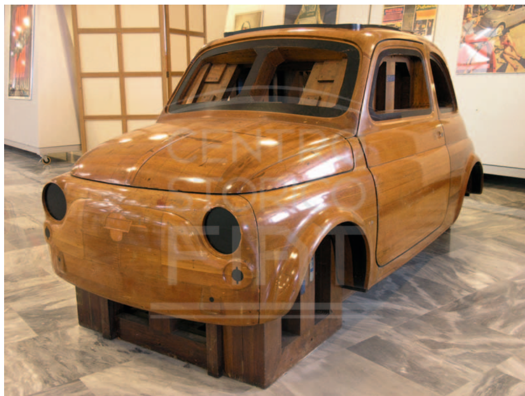
Master model for the coachwork dies of the Nuova 500. The master model is full-scale model of great accuracy made, at the time of the 600 and 500, in solid mahogany (later replaced by synthetic materials). It reproduced the form of all the surface accurate measurement point by point. This process is not so important now, following the arrival of new automatic plotter terminals attached to computers, making it possible to eliminate the manual plotting of sections.
