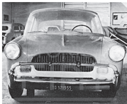
Full-scale plaster model made in 1955 (30 July), the year being shown on the number plate. A refinement of the previous 111 model, retaining its styling and curved lines. This model, never produced, would have been very similar to the models produced by Simca.
