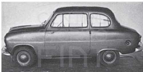
The prototype NSU-Fiat F05, also built at Heilbronn, with a two-cylinder water-cooled engine which incorporated components of the Fiat 1100 engine. This small car was also designed with front-wheel drive (1952-53).
