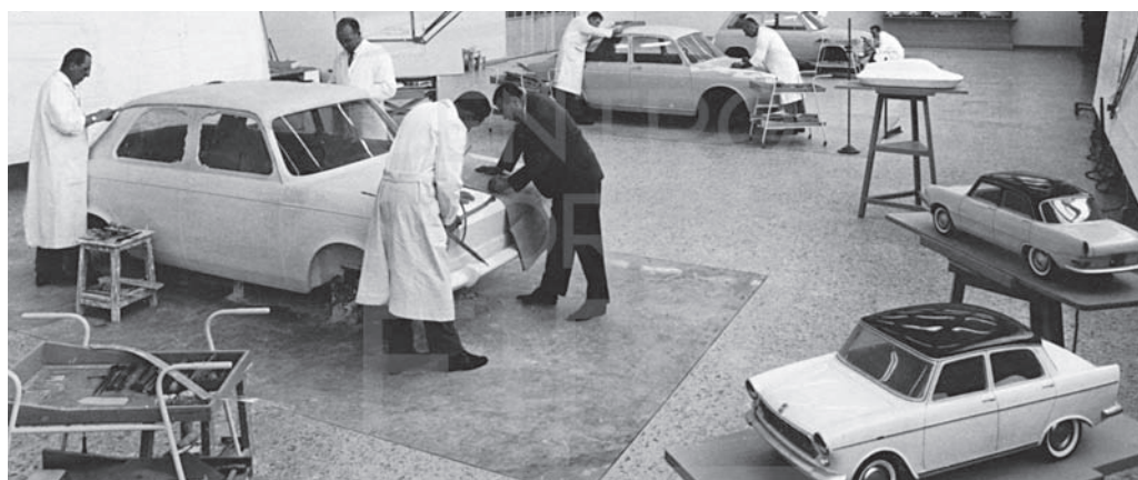
One of the large workshops for making plaster models at the Styling Centre in via La Manta (1962). In the foreground, one of the 1:5 models made during design exploration for the 1300-1500. Note the continued influence of the 1800 in the treatment of the roof panel and angularity of the body sides.
