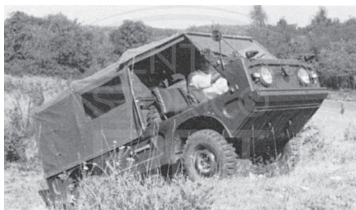
The experimental model 1120, not mentioned in the text, was designed to an idea of the author's by the Advanced Engineering Offices in 1959 and built in 1960 (completed in July). It was also nicknamed "Muletto". It could accommodate 5 passengers or 2 plus a load of 340 kg. In running order it weighed 580 kg unladen. The flat engine from the 500 estate supplied 23 hp and enabled it to do up to about 80 km/h and tackle gradients of up to 60°. It had independent drive on all four wheels and locking differentials. A magnificent off-road vehicle.
