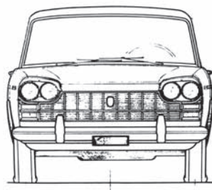
The final form of the front end of the 1800 and later the 2300 was the result of a long series of different efforts, the main stages being shown here. Note the characteristic eyelids over the headlights.
