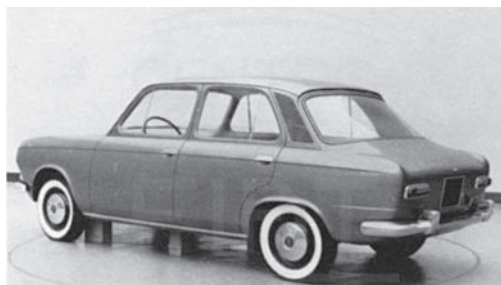
The coachwork of the G. 123 E2 was a compromise between two and three volumes. The rear position of the engine and the particular type of cooling allowed the front grille to be eliminated.
