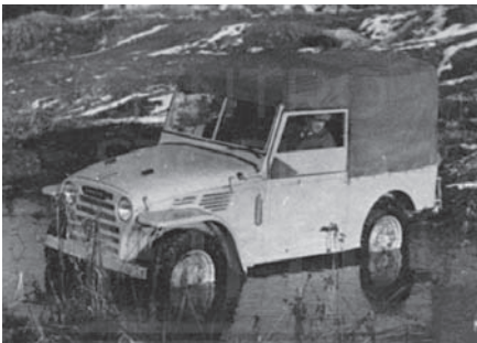
Carlo Salamano at a ford, testing a prototype of the Campagnola still fitted with a sloping engine-hood that was later redesigned.
