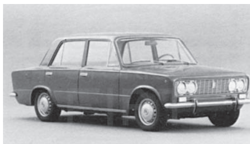
124 Special, unveiled on 6 October 1968, had an engine boosted from 1.197 to 1.438 cc, turning out 70 hp din.
