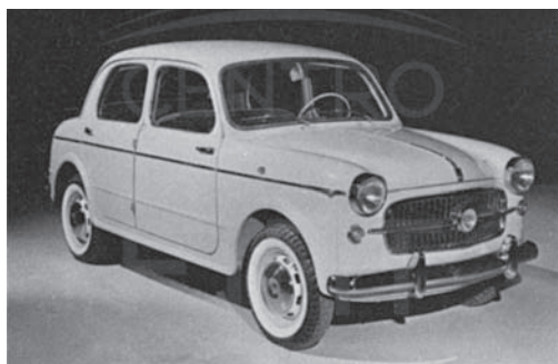
Standard 1100/103 E sedan (1956-57). In addition to some changes in styling, the auto's engine (103 E.000) had been redesigned and turned out some 10 % more power than the previous one.
