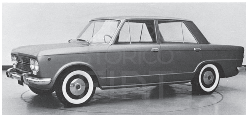
The 130 involved a whole series of full-scale plaster mock-ups. Size and styling were major concerns, made more pressing by the suggestions of the General Management. In the photograph: the first plaster mock-up, 1963.
