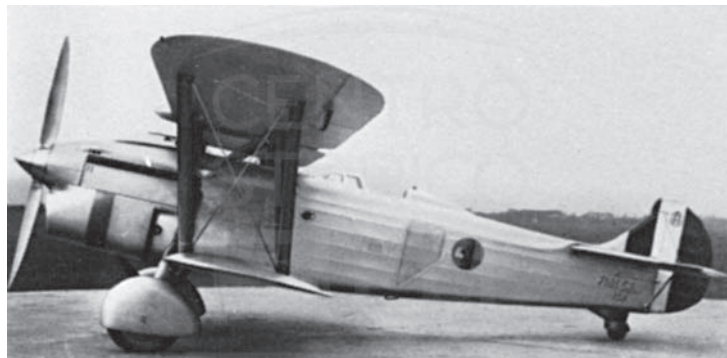
Fiat CR32 fighter-interceptor (1934), designed by Celestino Rosatelli. The airplane was fitted with an A 30 in-line engine.
