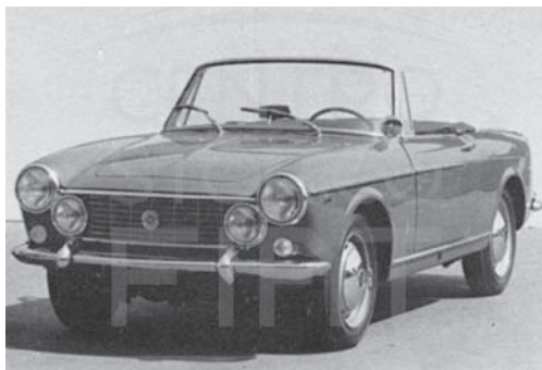
The final series of this cabriolet, called 1600 S from 1963 onwards, had a redesigned front and important modifications aimed at more flexible operation. Coachwork by the Pininfarina works.
