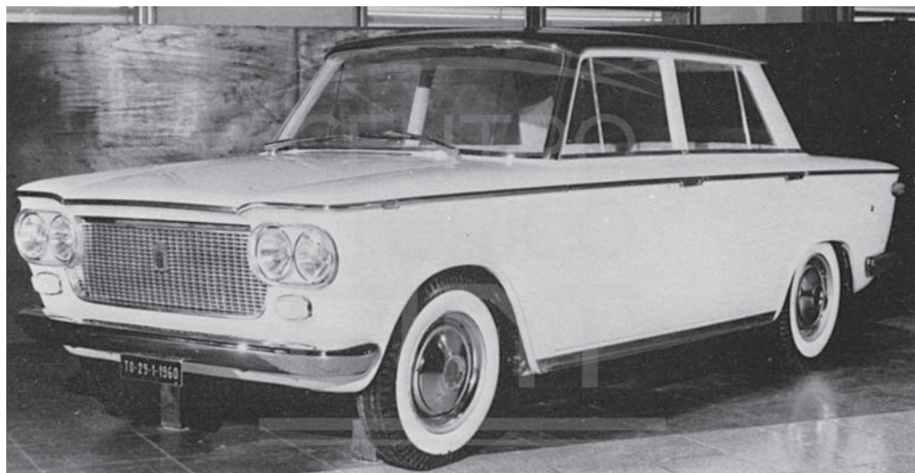
The final approved plaster model for the 1300-1500 drew strongly on the styling of the Chevrolet Corvair (and in turn probably influenced the NSU Prinz).
